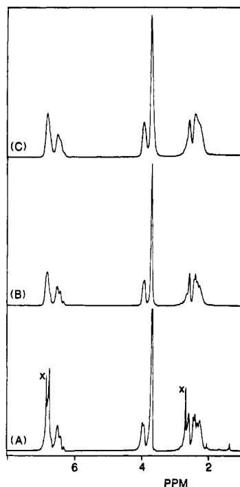
Figure 1. Concentration effects on the 500-MHz proton NMR spectrum of 50:50 mixtures of polystyrene and poly(vinyl methyl ether) at 65 °C. The solutions are (A) 1%, (B) 25%, and (C) 40% w/v in deuteriated toluene. The \times in spectrum A shows the residual toluene resonances.
